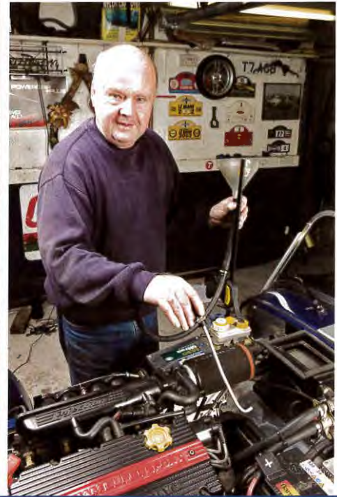
Fig 4: improvised devise for replenishing gearbox or diff oil: funnel, hose and angled pipe for oil delivery (see text).
